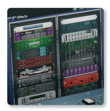
All effects processors and GEQs are custom-designed to function within this automatic latency compensation system. This ensures a phase-coherent, sample-accurate mix regardless of whether the devices are used as channel inserts or on auxiliary buses.
